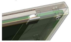
FFS Sensor $^{\text{TM}}$  integrated into 6mm thick display housing of a commercial flip phone
